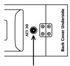
Alternatively, the MG-220 can be powered by an external 12Vdc source (such as car battery) connected via a 2.1mm DC jack located between the pistol grip and rear cover hinge. This jack is covered with a rubber plug for protection.
