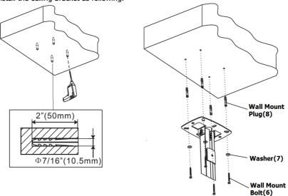
For Plastered ceiling installation first of all you need to find out where the wood stud is behind the ceiling using a stud finder. Then work out the position of the installation. While holding the ceiling mount against the ceiling use pencil to mark where the mounting holes will be and use an electric drill to drill a hole that is around 1/8" (3mm) wide and 2" (50mm) deep. Install the ceiling bracket as following.
