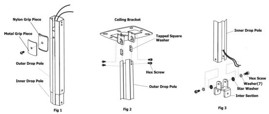
**Step 2** – Fixing Ceiling bracket
