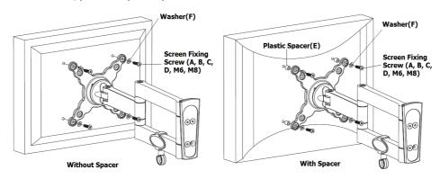
For VESA size bigger than 100x100, supplied adapter will allow bigger mounting VESA to fit up to 200x200. Please attached VESA extension arms as shown below using M5 12mm screw and nuts supplied.
